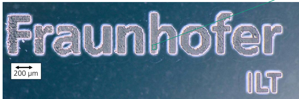
DIC image of transferred \mu LED-Array showing the "Fraunhofer ILT" lettering
