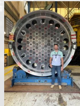
Graphite Core Block Shielding & Bulkhead
