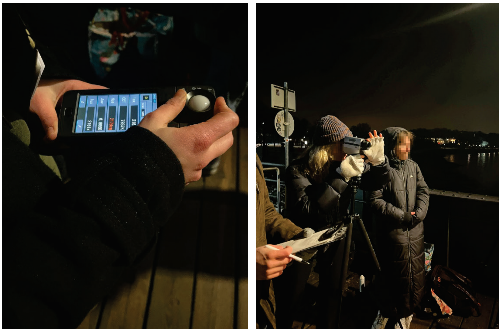
Fig. 4: Proof-of-concept measurements at Teufelsbrücker Platz, Hamburg, January 2023, Left: Using a chroma meter, Right: Measuring the luminance with a luminance spot meter, Credits: HAW Hamburg
