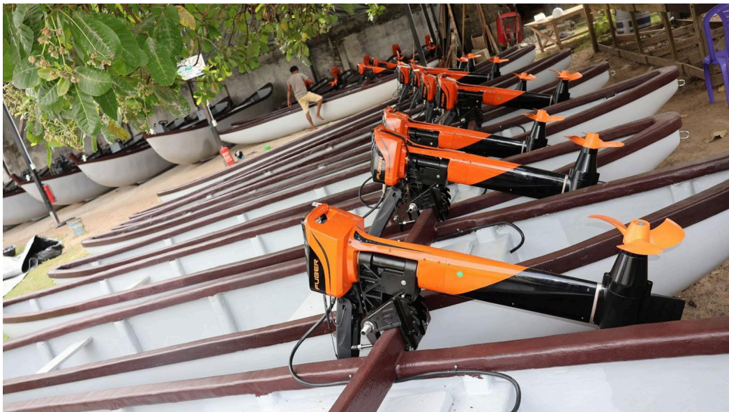
Solar Powered artisanal vessels -72 hours power on sea
