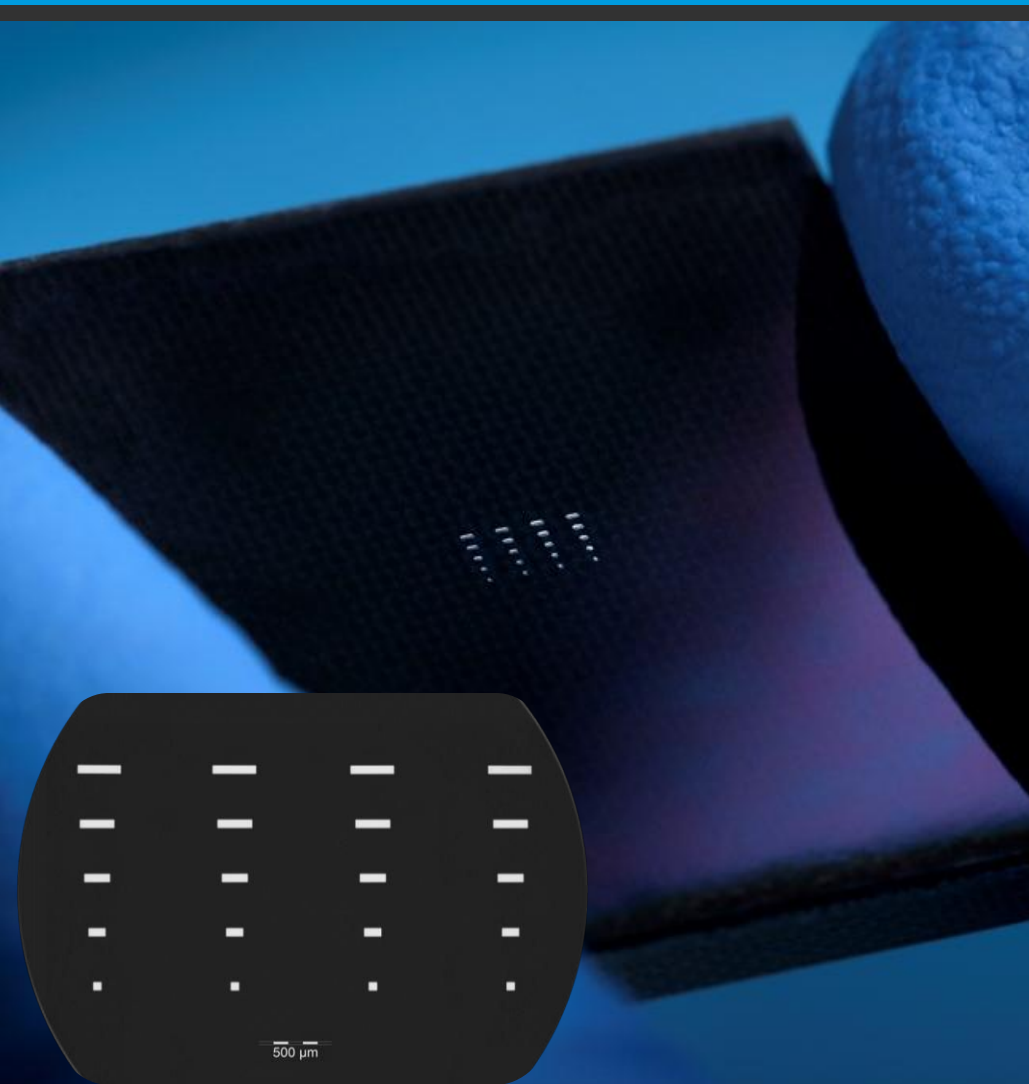
Maximum die size 300μm and AR of 5 (60×300 μm 2 )
