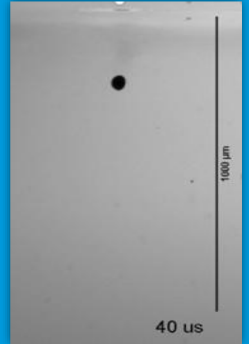
Real-time visualization snapshot (40µm dot of solder paste)
